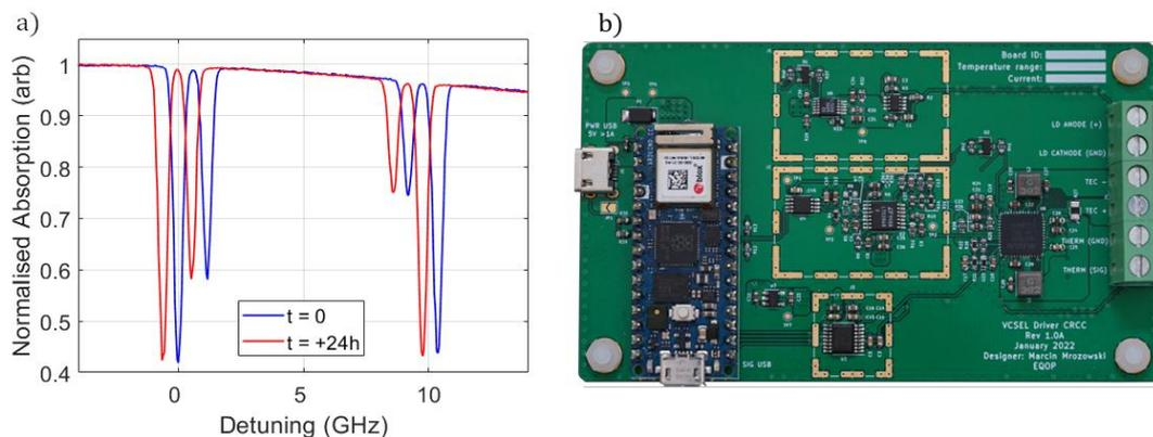
Figure 1: (a) Cs Spectroscopy 24 hour stability test. (b) Assembled device (dimension 100x60 mm) EMI shields removed to show internals.
