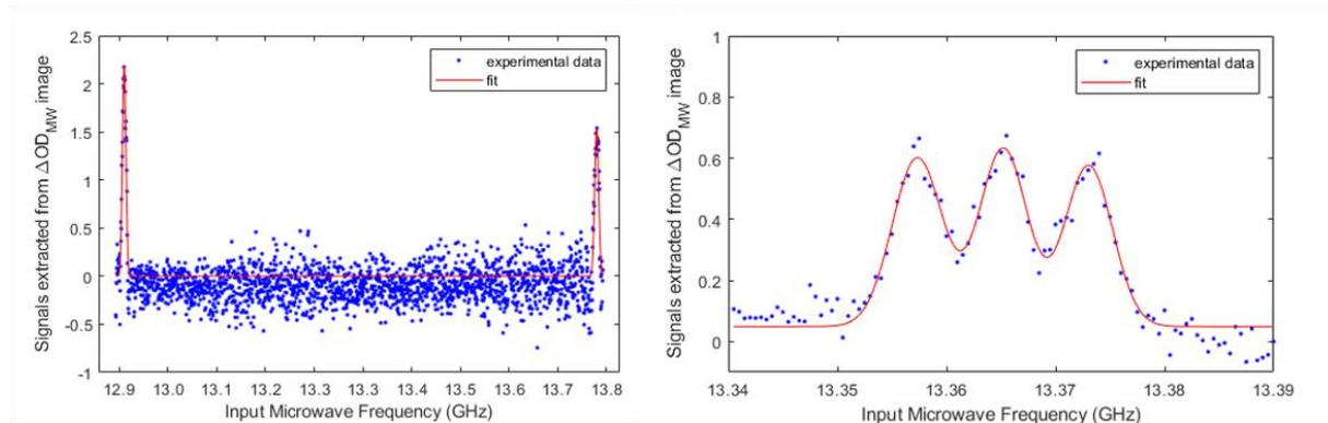
Figure 1: (Left) The measured instantaneous bandwidth is  $\sim 1$ GHz;
