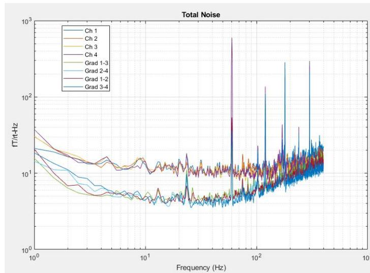
**Figure 1:** Magnetic sensitivity and gradiometric-inferred sensitivity of the four channels of the OPM module.
