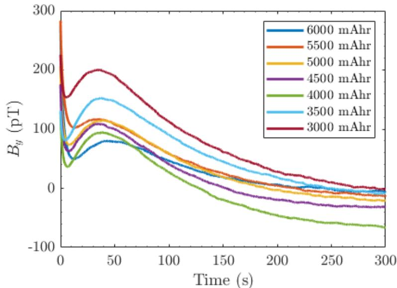
Figure 1: The magnetic field profile after a discharge cycle has finished at different states of charge for a single sensor in the 2x3 array.
