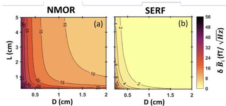
Figure 1: OPM intrinsic sensor sensitivity  $\delta \tilde{B}_i$  as a function of length  $L$  and width  $D$  of the sensing volume for NMOR (a) and for SERF (b)
