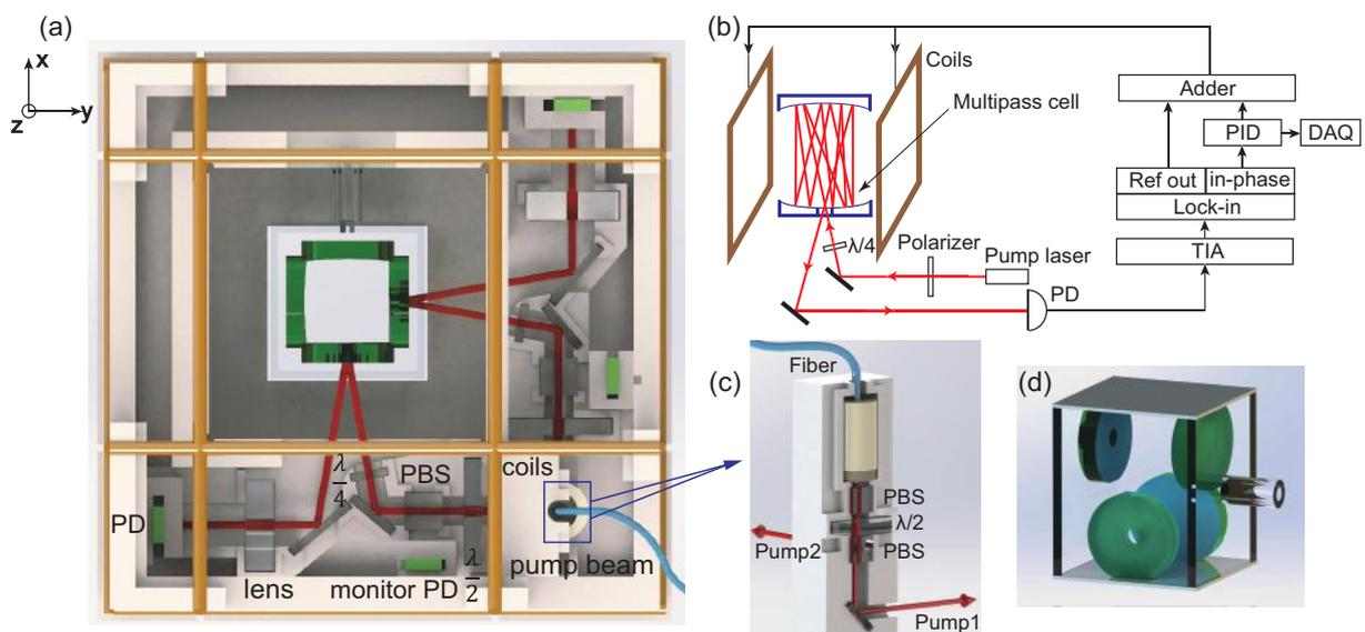
Figure 1: The vector atomic magnetometer setup.
