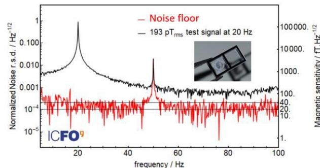
Figure 1: Magnetic noise measurement using a MEMS <sup>87</sup>Rb vapor cell and miniature biplanar coils – two components of a mass-manufacturable atomic magnetometer.
