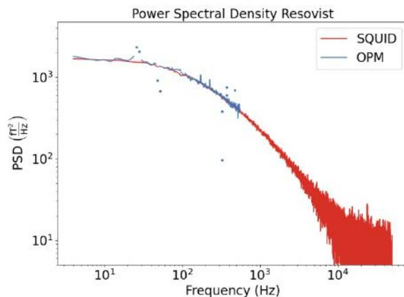
Figure 1: TNM spectra of a Resovist sample measured in the tabletop OPM setup and in an in house developed SQUID setup.
