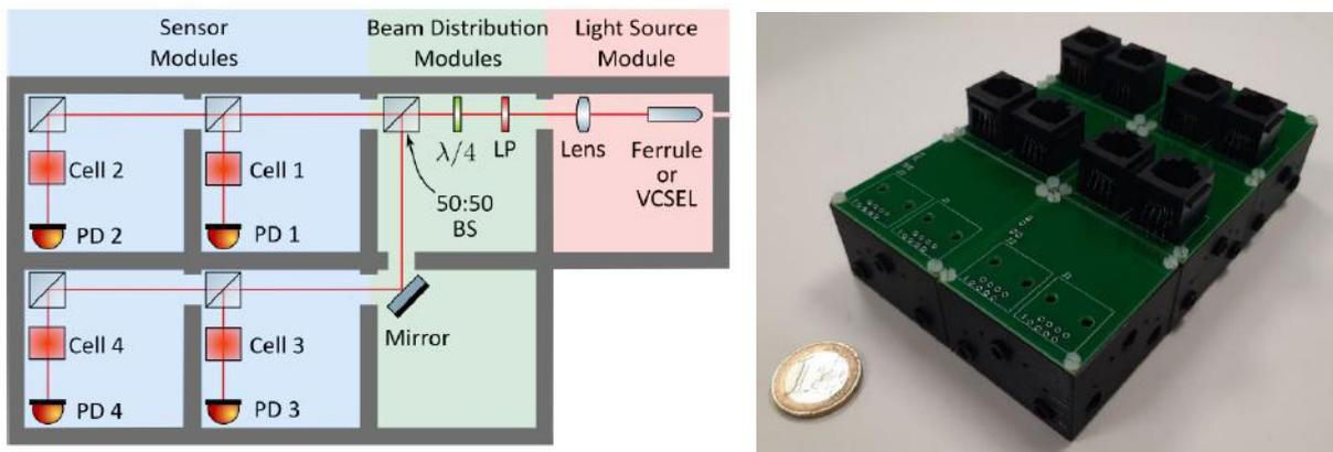
Figure 1: A schematic (left) [3] and photograph (right) of the modular OPM system, with a coin for scale. Modules can be easily snapped together to produce different configurations for various applications.
