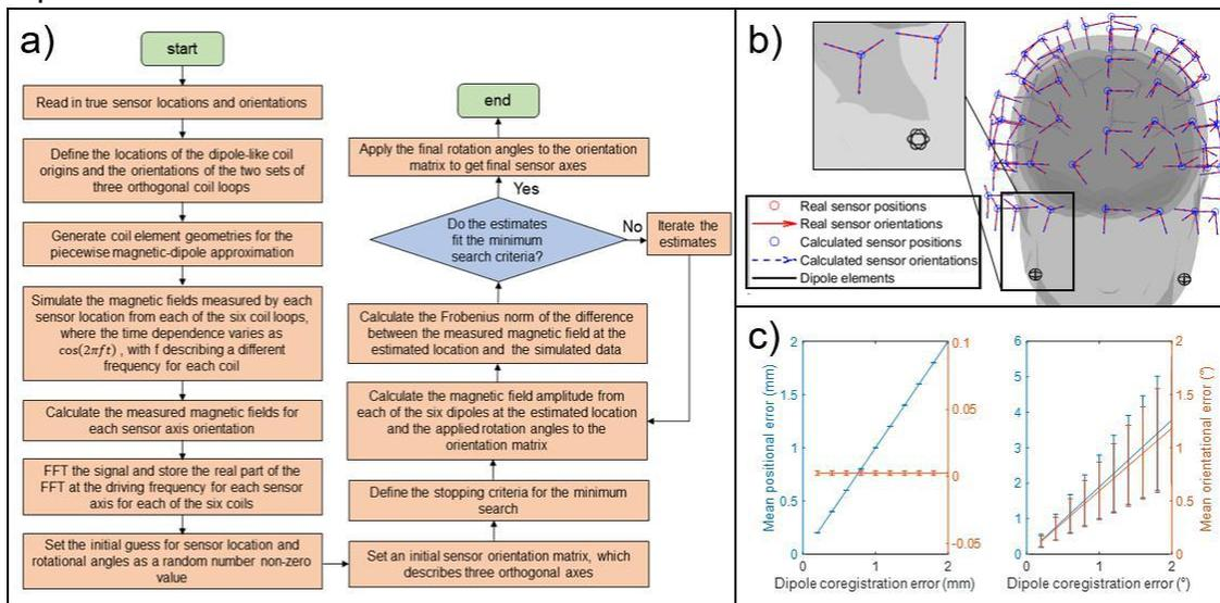
**Figure 1.** Figure 1a) flowchart describing how the algorithm determines sensor location and axes from simulated data. b) example co-registration on an MRI mesh. c) graphs of dipole coregistration error on calculated sensor position and orientation error.
