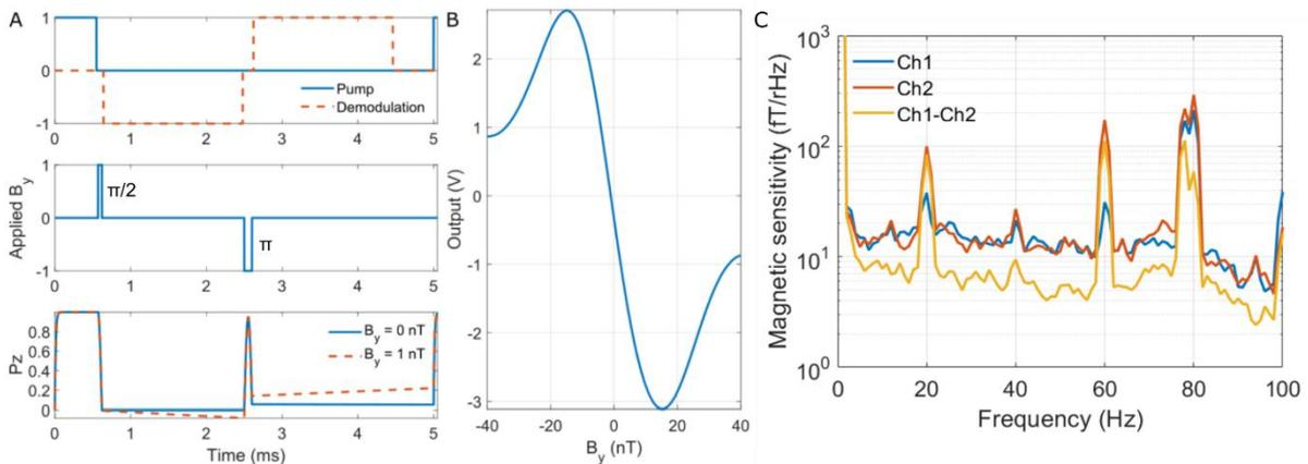
**Figure 1:** **A:** Pulse sequence for measuring the transverse field component  $B_y$  and the time-evolution of the spin polarization along the probe beam ( $P_z$ ). **B:** The demodulation output as a function of  $B_y$ . **C:** Magnetic and gradiometric sensitivity of two channels of the sensor.
