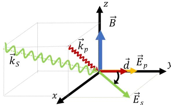
Figure 1: Excitation geometry for the detection of a single magnetic field component.
