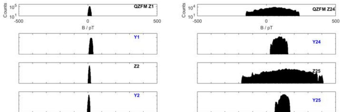
Figure 1: SERF-OPM signal histograms for (left) a 4-layer table-top shield (TwinLeaf MS-2), and (right) a two-layer magnetically shielded room with active compensation (VAC Ak3b).
