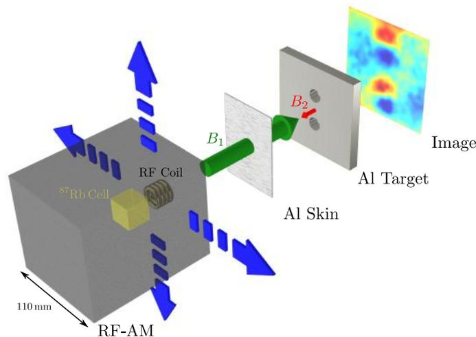
Figure 1: Illustrative depiction of the experimental geometry. A primary RF field  $B_1$  (green arrow) penetrates the Al skin and induces a secondary response field  $B_2$  (red arrow) in the target. The RF-AM is raster scanned across the geometry (blue arrows) building up an image of the magnetic response which reveals the structure of the target.
