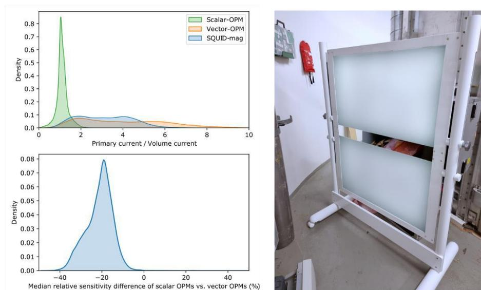
Figure 1: Top left: Ratio between primary and volume current contribution to measurements by scalar and scalp-normal-vector MEG systems. Bottom left: Relative sensitivity of scalar and scalp-normal-vector OPM measurements, across all background field directions. Right: Coil system for cancelling all homogenous and 1<sup>st</sup>-order gradient-field components, especially useful when operating in challenging magnetic environments.
