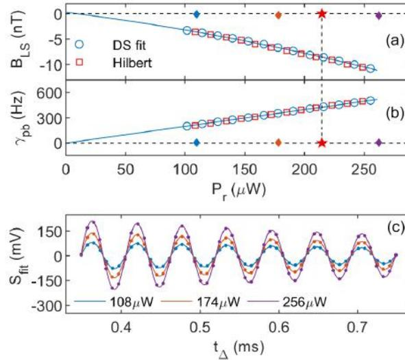
Figure 1: Suppression of (a) fictitious field  $B_{LS}$  and (b) power broadening  $\gamma_{pb}$  contributions using Ramsey-style interrogation. (c) Precession signals reconstructed with different readout powers. Variations in  $B_{LS}$  and  $\gamma_{pb}$  are represented as diamonds close to zero in (a) and (b).
