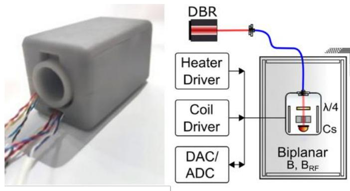
Figure 1: Left: Portable Sensor package with external dimensions of 25 x 25 x 41 mm (height, width and length respectively). Right: Experimental setup. Distributed Bragg reflector (DBR) laser (895nm), fibre coupled to portable sensor package, provides light that is polarised by a quarter waveplate ( $\lambda/4$ ), directed through a MEMs vapour cell, and detected by a photodiode.
