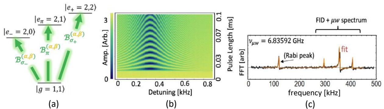
Figure 1: (a) MPE drives Rabi oscillations between  $F = 2$  and  $F = 1$  hyperfine manifolds.  $B_{\sigma_+}$ ,  $B_\pi$  and  $B_{\sigma_-}$  depend on direction  $(\alpha, \beta)$  of DC magnetic field. (b) Chevron Rabi pattern of  $\sigma_+$  transition. (c) Fit to the combined Larmor FID + microwave spectrum.
