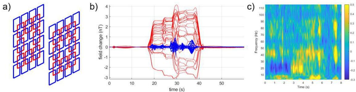
**Figure 1:** a) The matrix coil (b) Time-courses of data collected by an array of OPMs during a single up and go movement, blue/red shows data with/without coils. (c) Reconstructed neural oscillations associated with left index finger abduction (0-2s) and rest (2-8s) performed during continuous movement. Source reconstruction reveals the expected movement related decrease and post-movement rebound in the beta (13-30 Hz) band. Colour-bar shows change from baseline activity.
