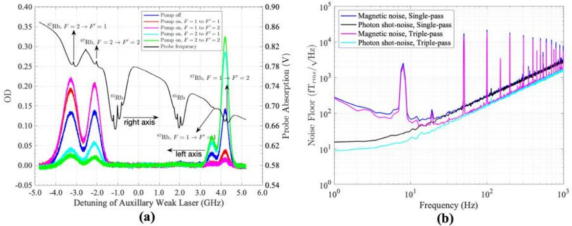
Figure 1: (a) Optical depth (OD) of <sup>87</sup>Rb atoms in the ground states under different pumping schemes and (b) sensitivity enhancement by using a triple-pass probe at a bias field of  $1.5 \mu\text{T}$ .
