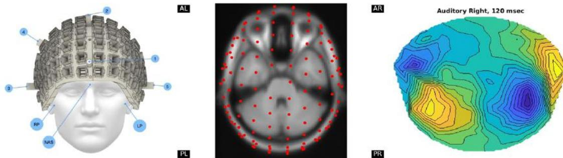
Figure 1: (left) Rendering of the OPM-MEG helmet and fiducials. (middle) Locations of the 120 OPMs overlaid on an MRI image. (right) Magnetic field map 120 ms after an auditory stimulation to the right ear of a subject.
