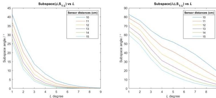
Figure 1: (Right) Signal errors  $\delta\Phi$  have higher subspace angles with vector spherical harmonic basis truncated at the  $L^{\text{th}}$ -degree ( $\mathbf{S}_{1:L}$ ), and requires higher  $L$  truncation to explain when compared to the true signal  $\Phi$  case (left). This means  $\delta\Phi$  contain higher-frequency components with higher errors than  $\Phi$ .
