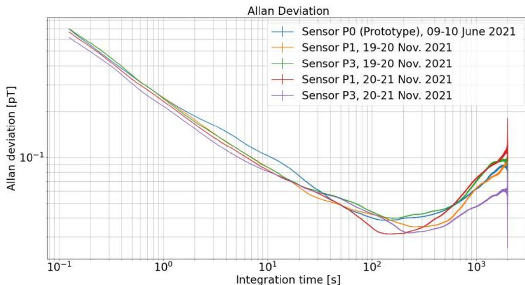
Figure 1: Allan standard deviation of measurements taken with different sensors on various days. All measurements show a stability below 50 fT between 70 and 600 s.
