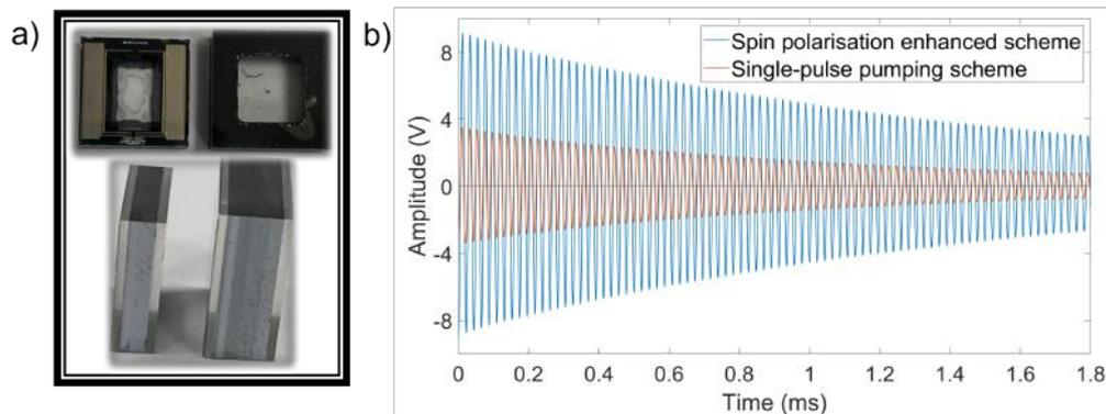
Figure 1: a) Left: previous 1.5 mm thick Cs MEMS cell fabricated at Texas Instruments. Right: 3 mm cell produced at Kelvin Nanotechnology in collaboration with UoS. b) Improved FSP signal achieved through more efficient optical pumping which enhances the spin polarisation buildup.
