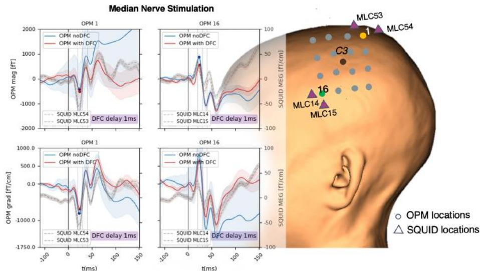
Figure 1: OPM responses to median nerve stimulation with and without DFC (red and blue, respectively). Selected SQUID MEG sensor responses are shown in gray.
