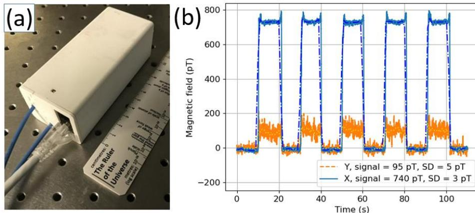
Figure 1: (a) Prototype OPM. (b) Magnetometer signal when a 3 cm aluminium disk is placed near the OPM at  $t = 10$  s and then removed again at  $t = 20$  s (5 repetitions).
