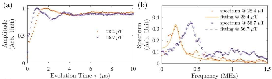
Figure 1: Sodium ground-state free-precession detected with ASE. (a) ASE intensity as a function of the evolution time. (b) Fourier transform of the ground-state free-precession.
