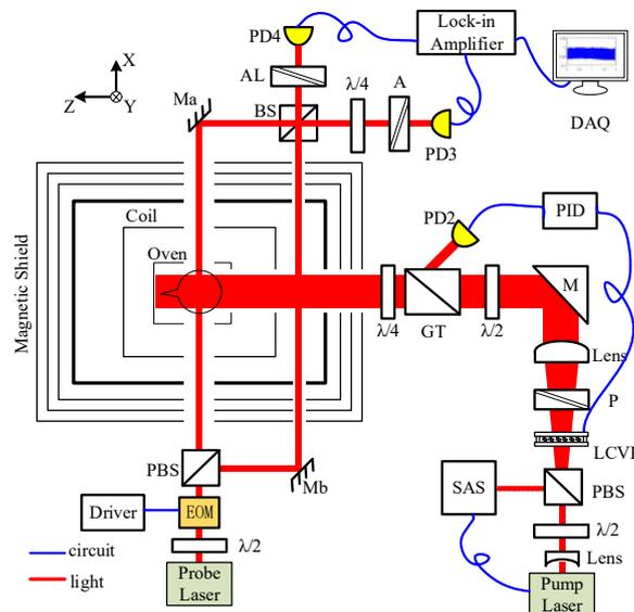
Figure 1: Schematic of experimental setup. EOM: electro-optic phase modulator, PBS: polarizing beam splitter, BS: beam splitter, M: mirror, A: analyzer, PD: photodiode, DAQ: data acquisition system. LCVR: liquid crystal phase retarder, GT: Glen Taylor prism. P: polarizer,  $\lambda/2$ : half wave plate  $\lambda/4$ : quarter-wave plate SAS: Saturation absorption module
