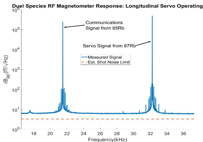
Figure 1: Preliminary data from the operation of our dual species magnetometer with longitudinal feedback engaged, demonstrating our ability to servo the magnetic field using <sup>87</sup>Rb whilst simultaneously detecting a communications signal from <sup>85</sup>Rb with good noise performance.
