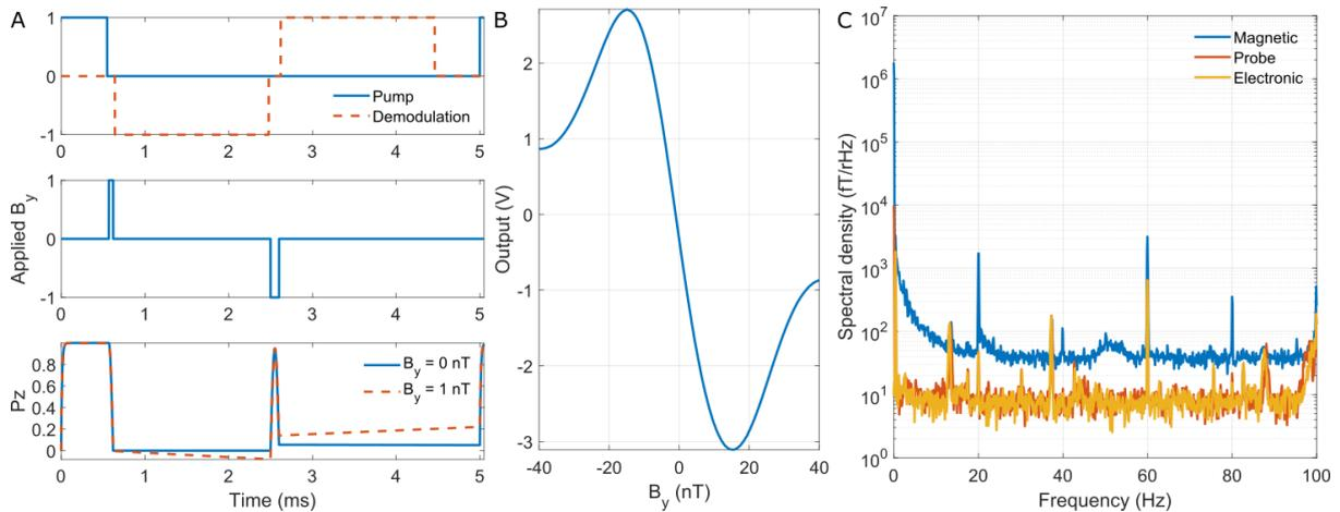
**Fig. 1 A:** Pulse sequence for measuring  $B_y$ . Top two panels illustrate the pump signal, demodulation waveform and the magnetic field pulses along the y-axis while the bottom panel shows the time-evolution of the spin polarization along pump/probe beams. **B:** Measured signal after demodulation as a function of  $B_y$ . **C:** Noise spectral density. Magnetic noise is shown as well as the estimated noise contributions from the probe beam and electronics.
