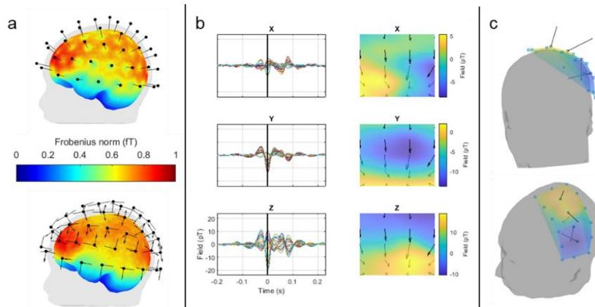
Figure 1: a) A simulated triaxial array (bottom) results in more uniform coverage, compared to a radial-only array (top). b) MCG signals measured with triaxial sensors. c) Vector neuromagnetic fields from 4 triaxial OPMs placed over left primary sensorimotor cortex.
