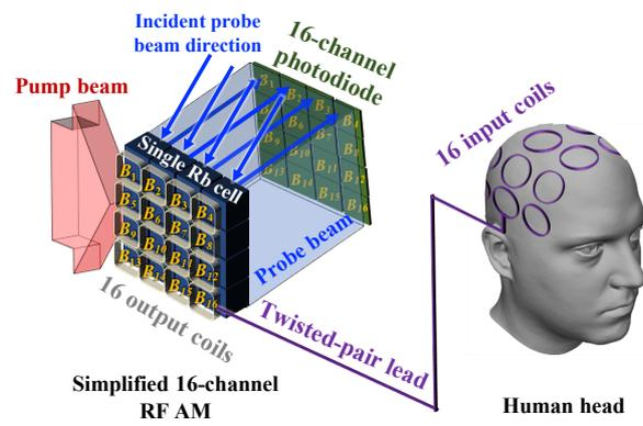
Figure 1: Illustration of the multi-channel OPM parallel ULF MRI device.
