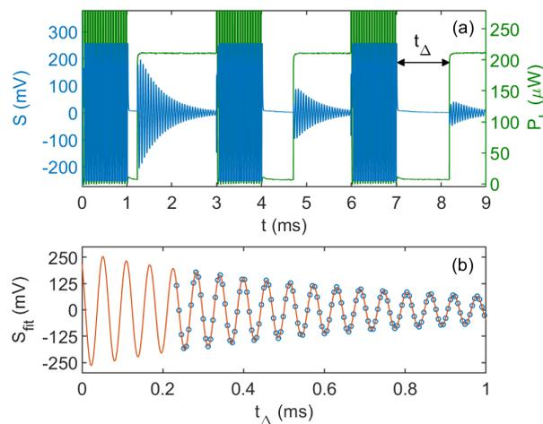
Figure 1: (a) FID signal train subsection, and corresponding laser power prior to illuminating the vapor cell which is set close to zero for a time,  $t_\Delta$ , after optical pumping. (b) Reconstructed precession signal exhibiting spin dynamics unperturbed by the  $210 \mu\text{W}$  readout field.
