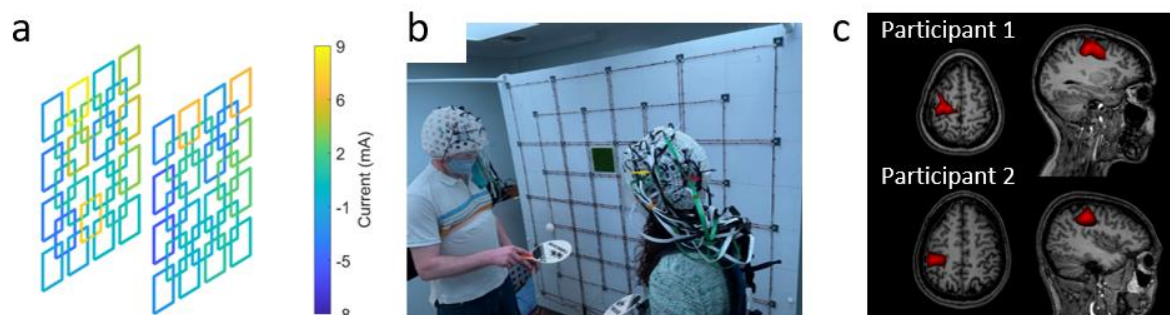
Figure 1: OPM-MEG scanning of real-time interactions. a) The 48-coil bi-planar matrix coil system. The current in each coil is individually controlled to generate the required field in order to cancel the remnant magnetic field inside the MSR. b) Two participants each held a table-tennis bat in their right hand and hit the ball back and forth to each other; a 5 s rally was followed by 7 s rest. c) The spatial pattern of measured data suggests activation in the sensorimotor regions during the rally.
