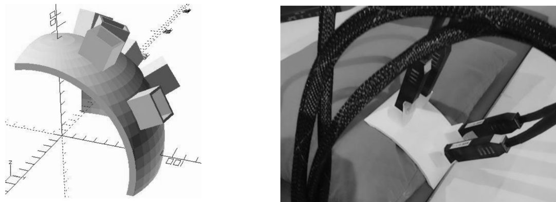
Fig. 1 (left) Schematic 3D design for the generative manufacture of an MEG OPM sensor array holder. (right) Picture of the four channel MCG holder.
