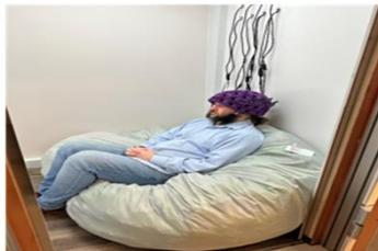
Figure 1: OPM-MEG setup in magnetically shielded room. Subject is seated but the head is free to move.
