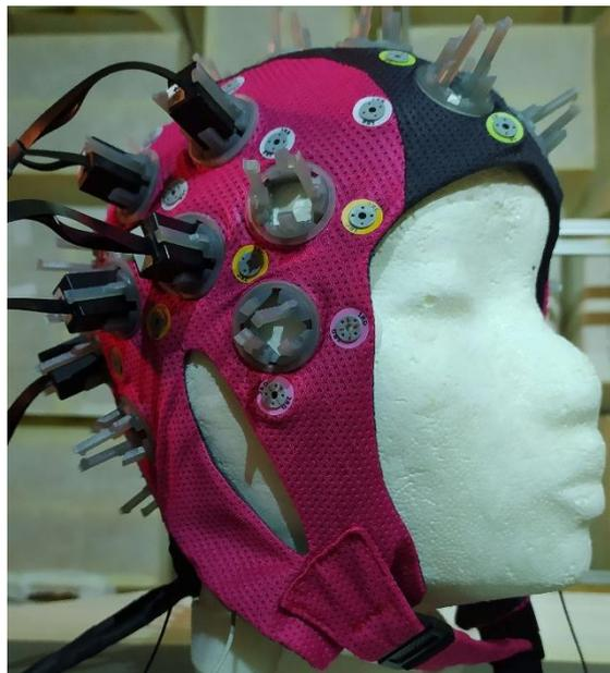
Figure 1: Textile cap for simultaneous EEG and OPM-MEG measurements.
