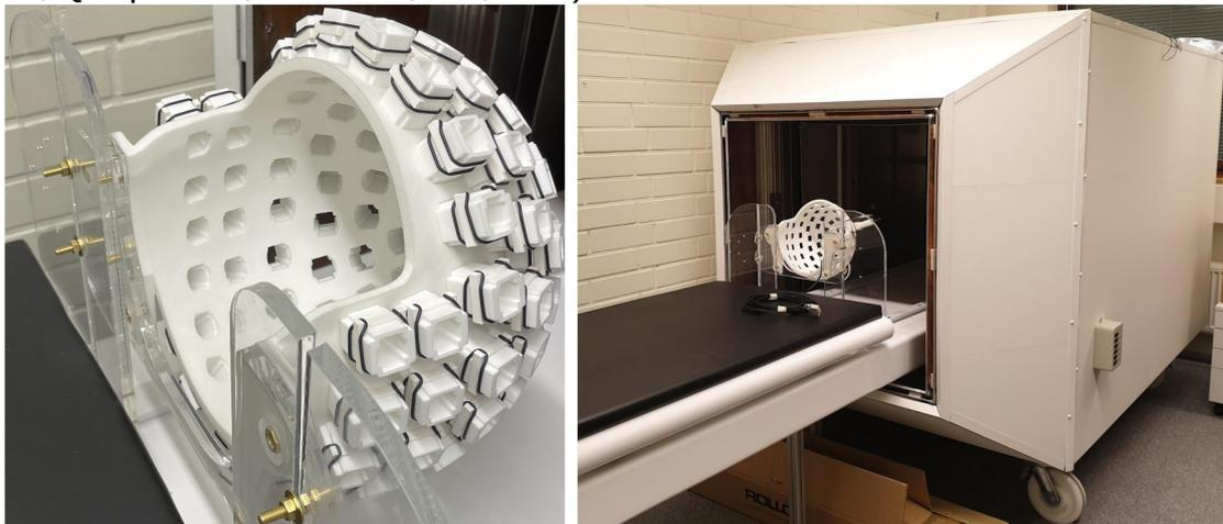
Figure 1: OPM sensor helmet and compact person-sized shield.
